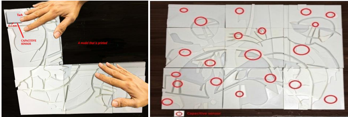
Figure 5: The appearance of a capacitive sensor (left) and 3D printed model with the locations of the capacitive sensors (right)
